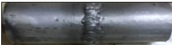
Fig. 1: Sample of MIG Welded pipe (3 mm/min)
